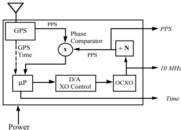
**Figure 4. Second-Generation GPS Clock**
