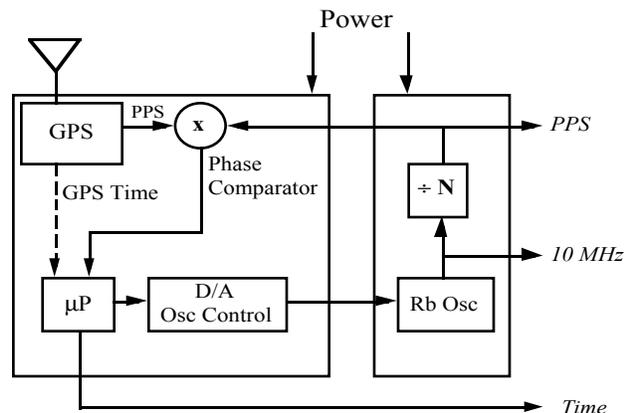
**Figure 3. First-Generation GPS Clock**
