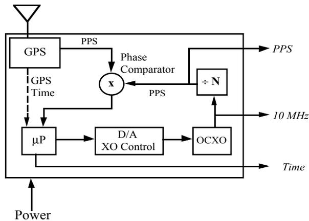
**Figure 4. Second-Generation GPS Clock**
