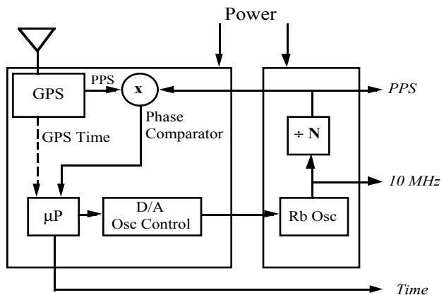
**Figure 3. First-Generation GPS Clock**
