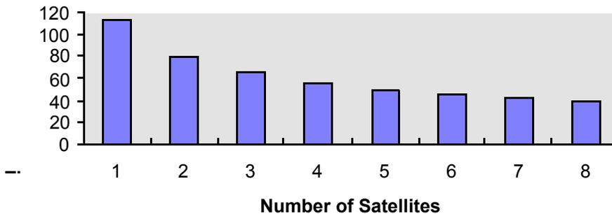
almost one part in  $10^{10}$ . A multi-channel GPS receiver can average the SA errors over seven or eight satellites if clear view of the sky is available, reducing the effect of SA by almost a factor of three (Figure 2).
