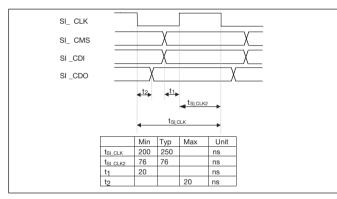
Figure 8. Timing diagram of the serial interface.
