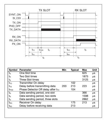
Figure 6 and table 2. Timing sequence for data transmission.
