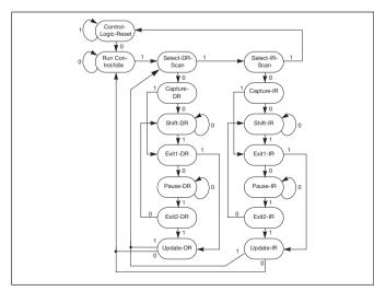
Figure 9. State machine for serial interface control. '0' denotes a logic level 'low' and '1' level 'high' level on the SI\_CMS control pin.
