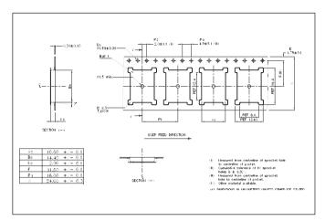
Figure 15. Carrier tape dimensions.
