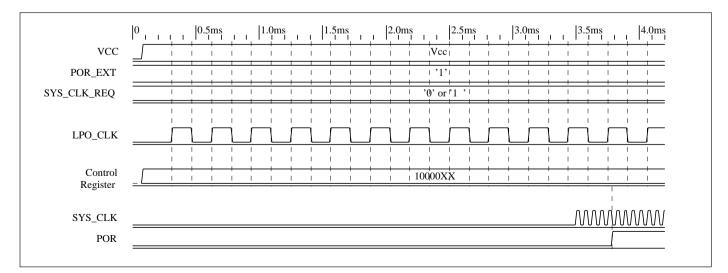
Figure 7. Powering up the module.
