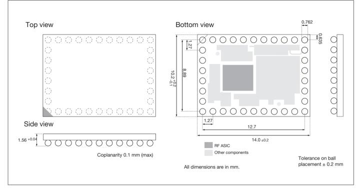
Figure 4. Mechanical dimensions of PBA 313 01.
