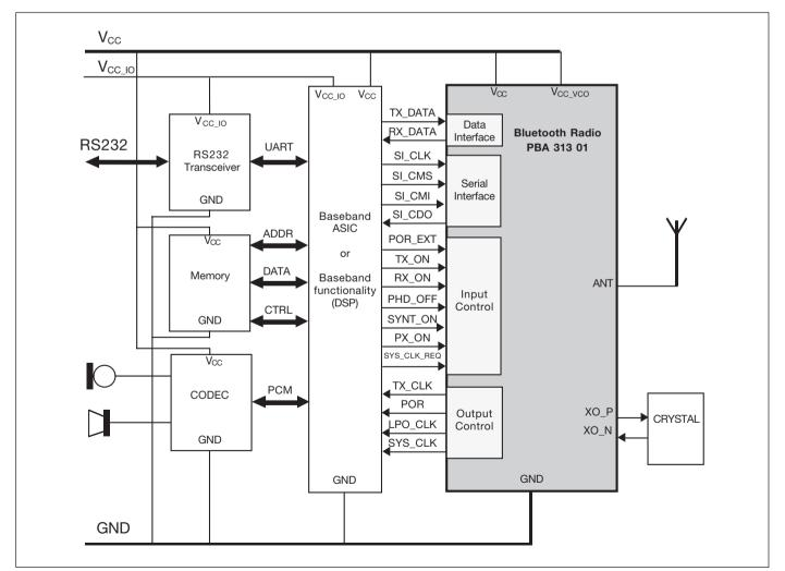
Figure 11. Typical UART or PCM configuration.
